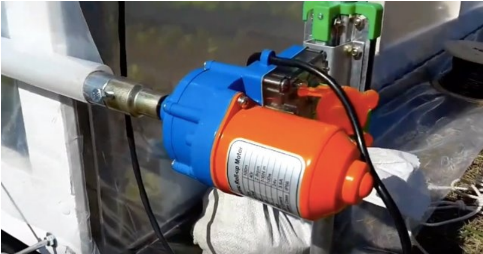
Image 62: Close-up of a roller motor that can roll up the tarpaulin of a tunnel greenhouse
