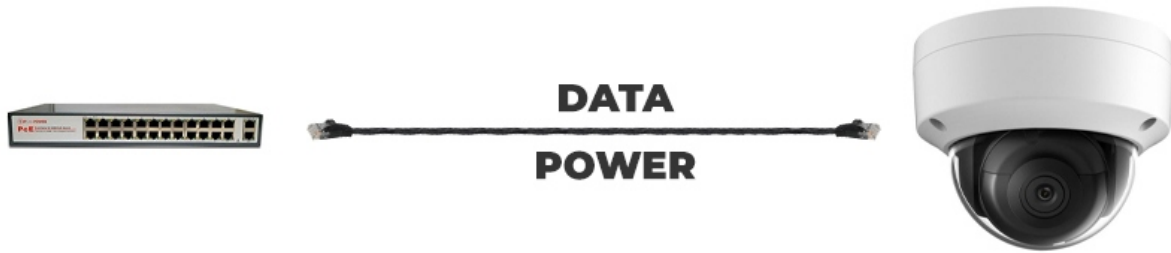
Image 11: Power over Ethernet application with a camera
