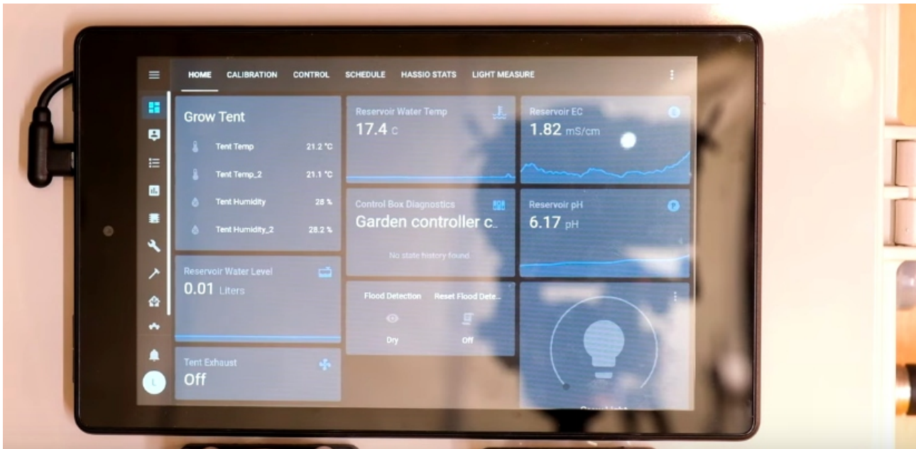
Image 16: Dashboard using software package Home Assistant, as applied by the youtuber LED Gardener 8 . Opened here on a tablet.
