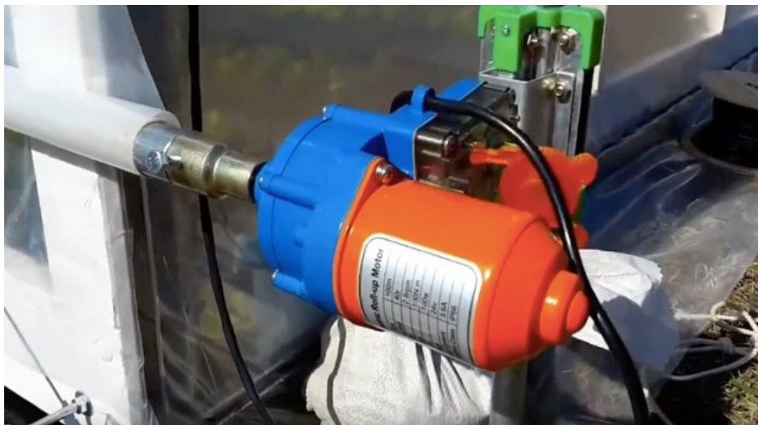
Image 43: Close up of a roller motor that can roll up the tarpaulin of a tunnel greenhouse
